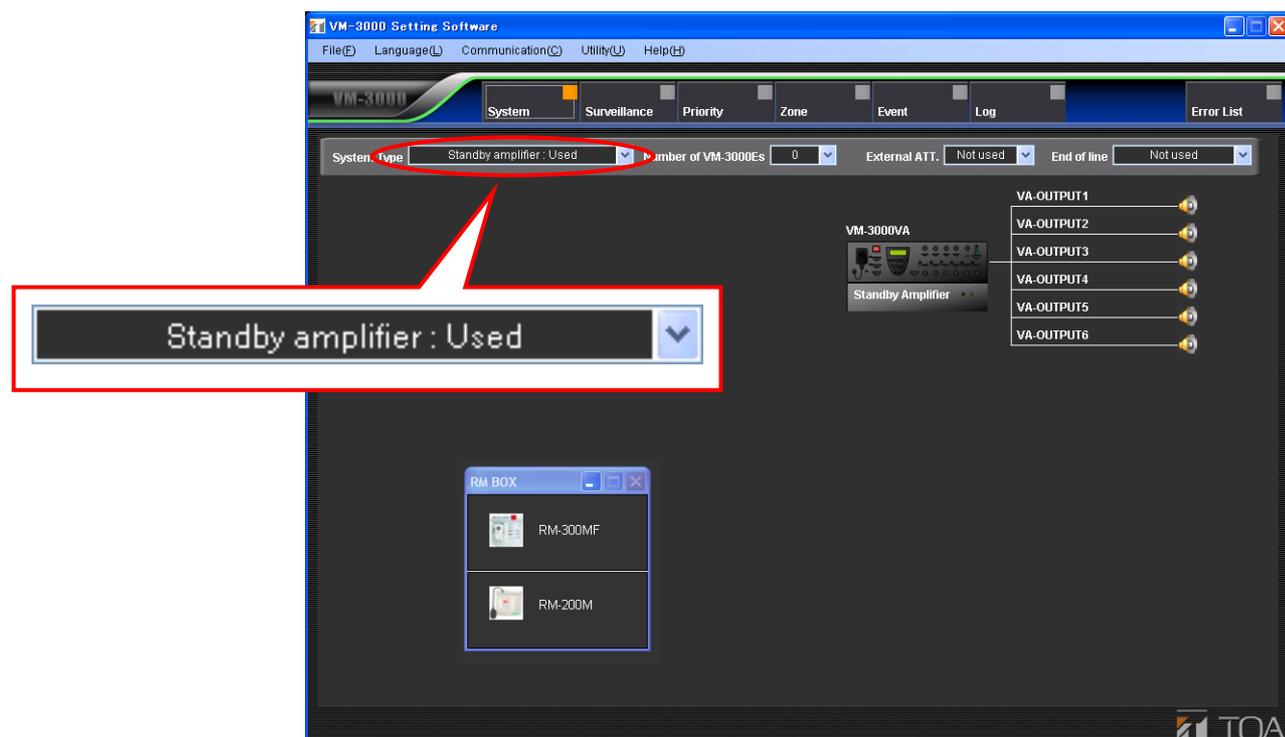
Setting this to "BGM/Paging System" allows connection of a VP-2000 series amplifier to each VM-3000VA and VM-3000E in order to configure simultaneous 2-channel broadcast system for BGM and paging announcement.
