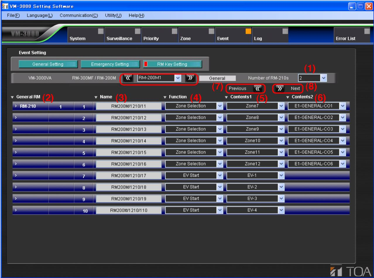
Click the "RM-300MF/RM-200M" selection box or double-arrow button to select the RM-300MF or RM-200M. The display switches to the screen for setting the selected device.
