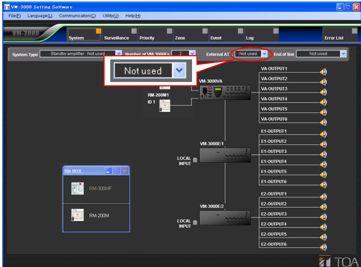
Setting this to "All output" causes the speaker lines to be displayed as shown at right.
