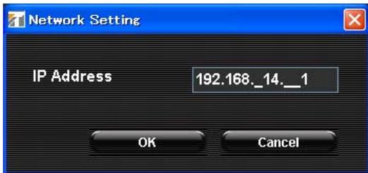
**Step 2.** Set the VM-3000VA's IP address. (Default IP address: 192.168.14.1)
