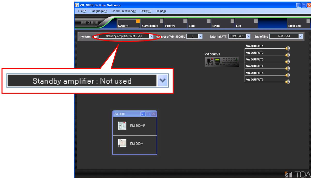
Setting this to "Standby amplifier: Used" sets the configuration to a system that does use a standby amplifier. In such cases, use a VP-2000 series amplifier as the VM-3000VA's standby amplifier.
