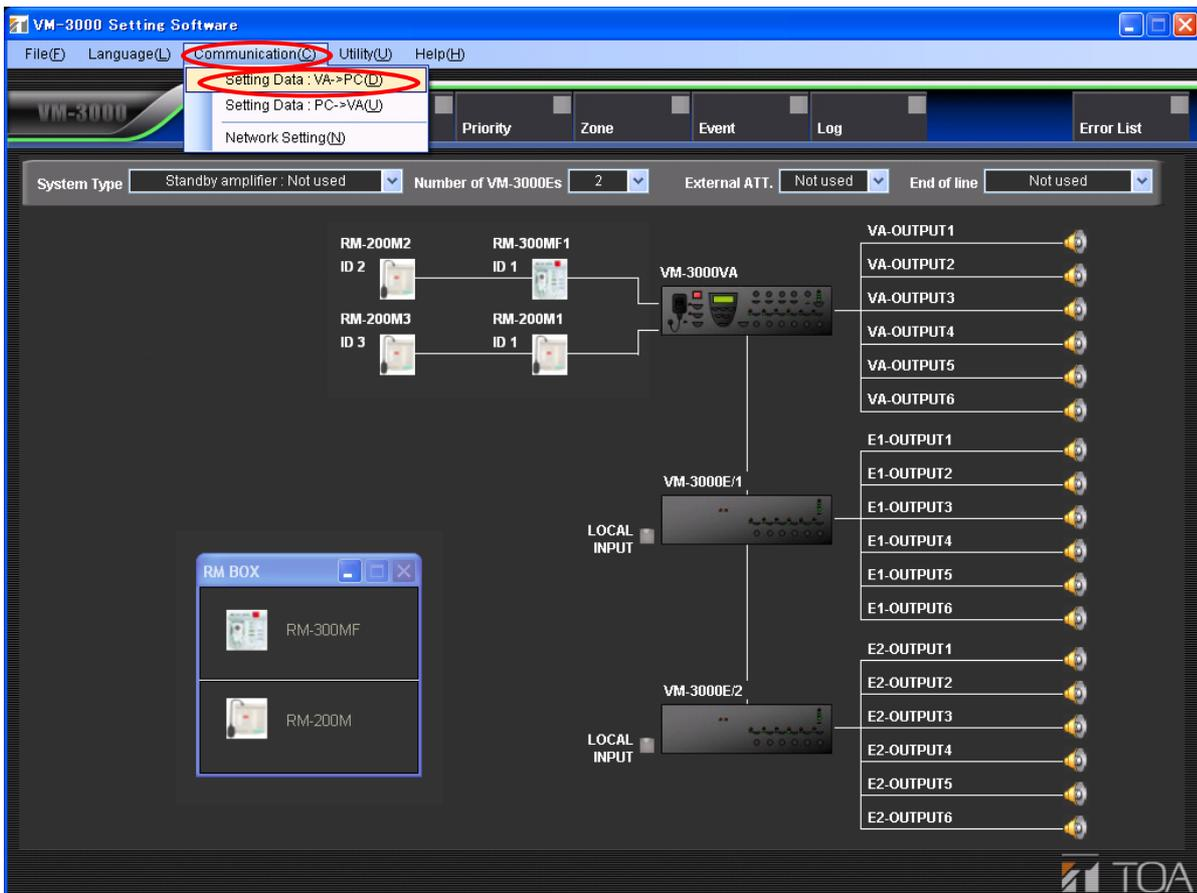
The transferred setting content is displayed on the current setting screen when the data has been transferred. In this event, the VM-3000VA's LCD screen displays as follows:
