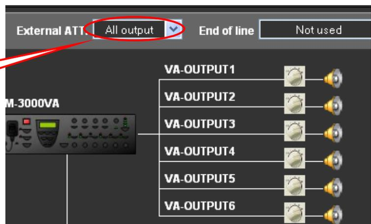
Setting this to "Each output" causes the speaker lines to be displayed as shown at right.
